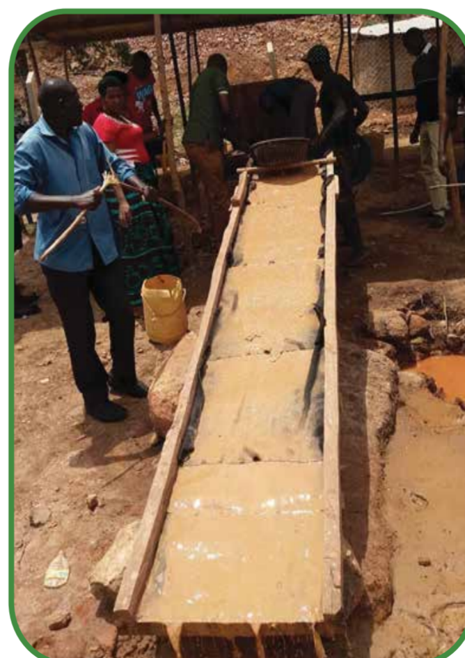
Sluicing to separate by gravity
